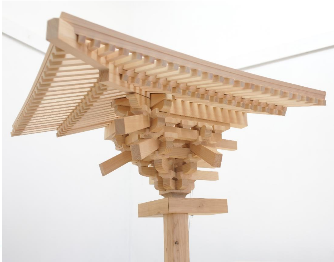
Model comprising assembled processed parts by robots (roof corner, 1/5 scale)
